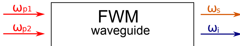
Figure 1.5: Schematization of a four wave mixing process: the two different pump photons are injected from the facet of the waveguide and are subsequently converted into the signal and idler frequencies.
